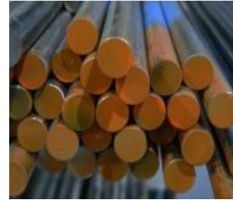
Alloy 625 Annealed Condition ASTM B446-03
